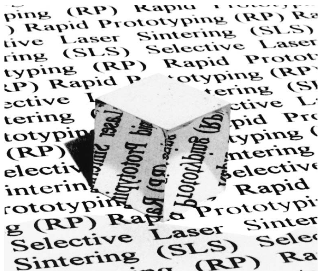
Figure 8 Polished cube of 316L stainless steel material. Density measured at >99.5%.
